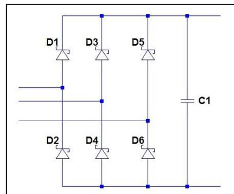
into the top common wire and negative power pushed into the common bottom line, or ground. With two diodes on each phase, the positive power of each AC phase is sent to a common line (top line). With each phase being 120° (or one-third) out of phase with the other lines, this creates an average single-phase power.
