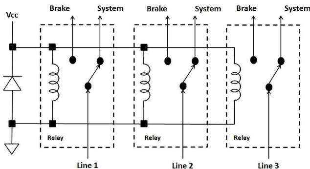
The braking system is a set of three relays, each of which is connected to one phase of the generator and act as a switch to toggle the path of incoming power. Each relay has a main input line that is connected to one of two output pins. When an internal coil is energized, the switch that connects the input with one output toggles
