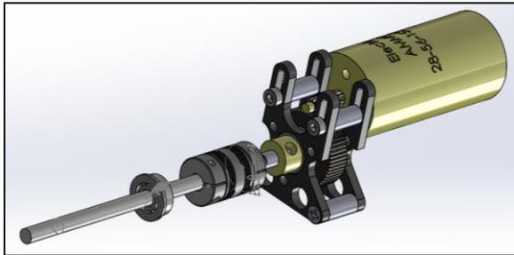
The rotational movement developed by the rotor is transferred to a small steel shaft that is connected to the gearbox with a flexible helical coupler. The coupler is essential to the safe operation of the wind turbine because it absorbs the vibrations and external forces from the rotor before they reach the gearbox or generator. This will increase the lifetime of these components while effectively transferring power to the generator.
