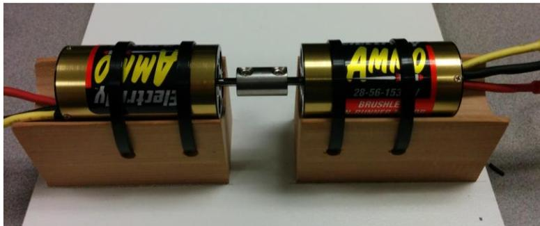
**Figure 7. Controllable Motor Test Setup**
