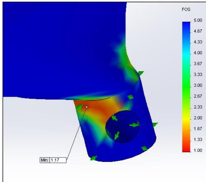
Figure 5. Initial FEA performed on original blade design at 4000 RPM and 0.1 s braking time
