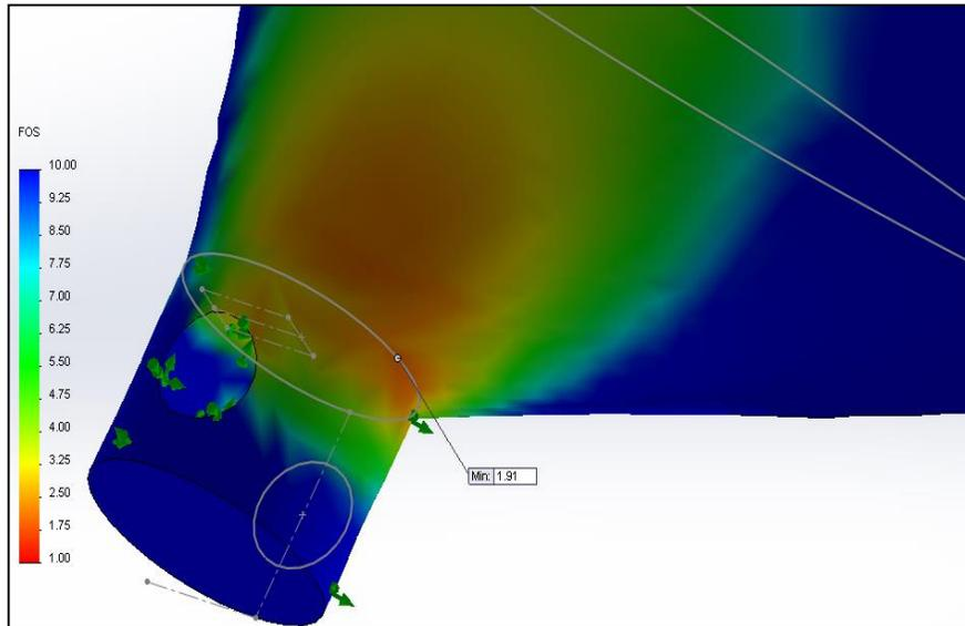
Figure 6. FEA results after redesign. RPM = 4058 and stopping time = .1 seconds.
