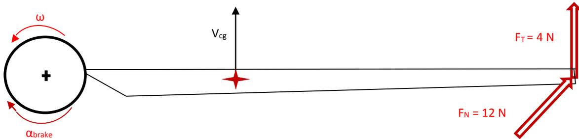
Figure 4. FBD of single airfoil. This diagram shows the placement of the loads for FEA modeling.
