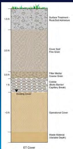
Figure 7.3-5 Cross-section of ET cove
