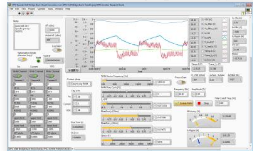
Physical and FPGA-simulated waveforms after global optimization of (Vce, Ron, L, R_LESR, R_BATCharge, R_BATDischarge)
