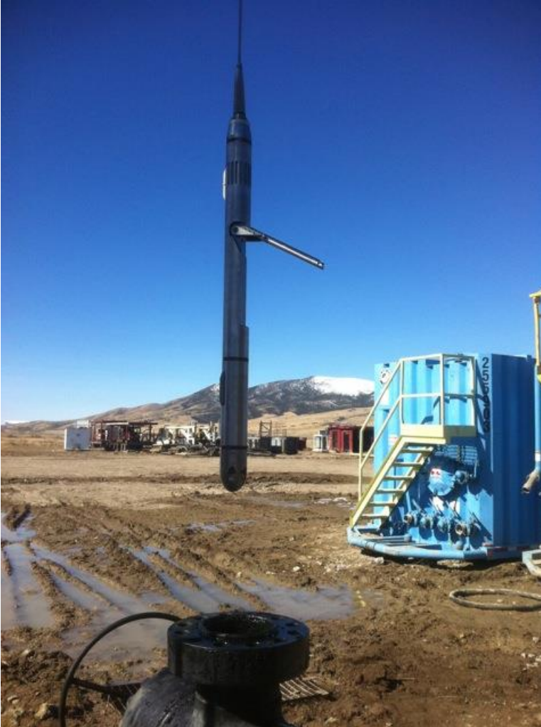
Deployment of Calidus 200 C, 3-C Tool at Raft River ( Japanese tool and LBNL wireline truck)
