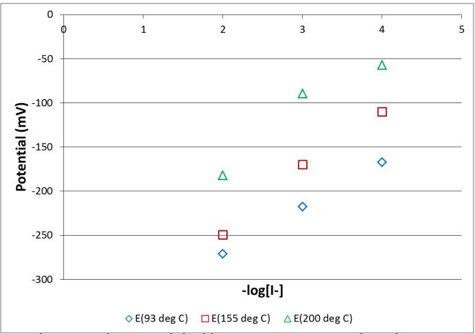
We see an increase in potential with temperature at a given I concentration which agrees with electrochemical theory
