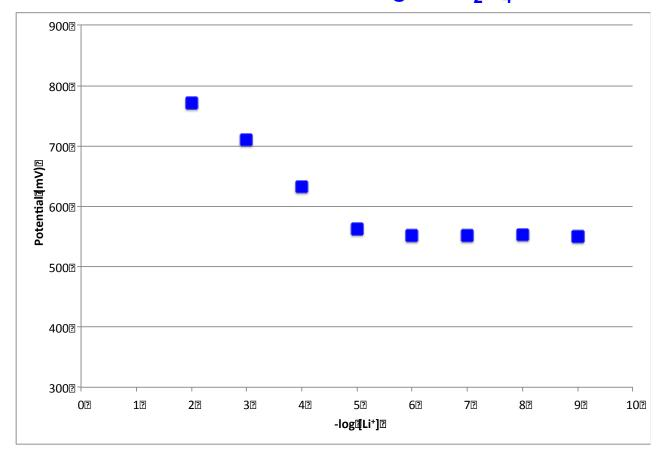
Slope in the 10<sup>-5</sup> to 10<sup>-2</sup> M region = -70.6 mV/decade Limit of Detection: 10<sup>-5.15</sup> M in 0.1M NaCl-KCl
