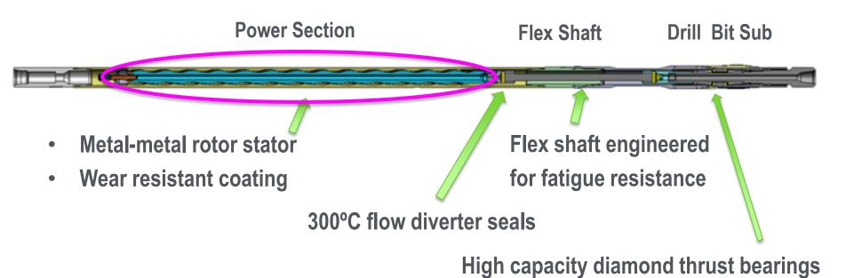
for high weight on bit hard rock drilling
