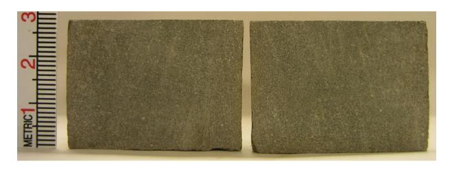
Three week cure in brine/ $CO_2$ . Right sample is treated with phenolphthalein. No color change indicates pH < 10.
