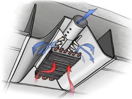
Figure 2: Active Chilled Beam Design
