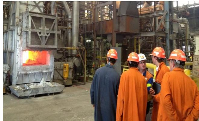
University of Dayton and University of Kentucky IAC students evaluate the operation of a large reverb aluminum melt furnace located at a smelting facility in Kentucky.
