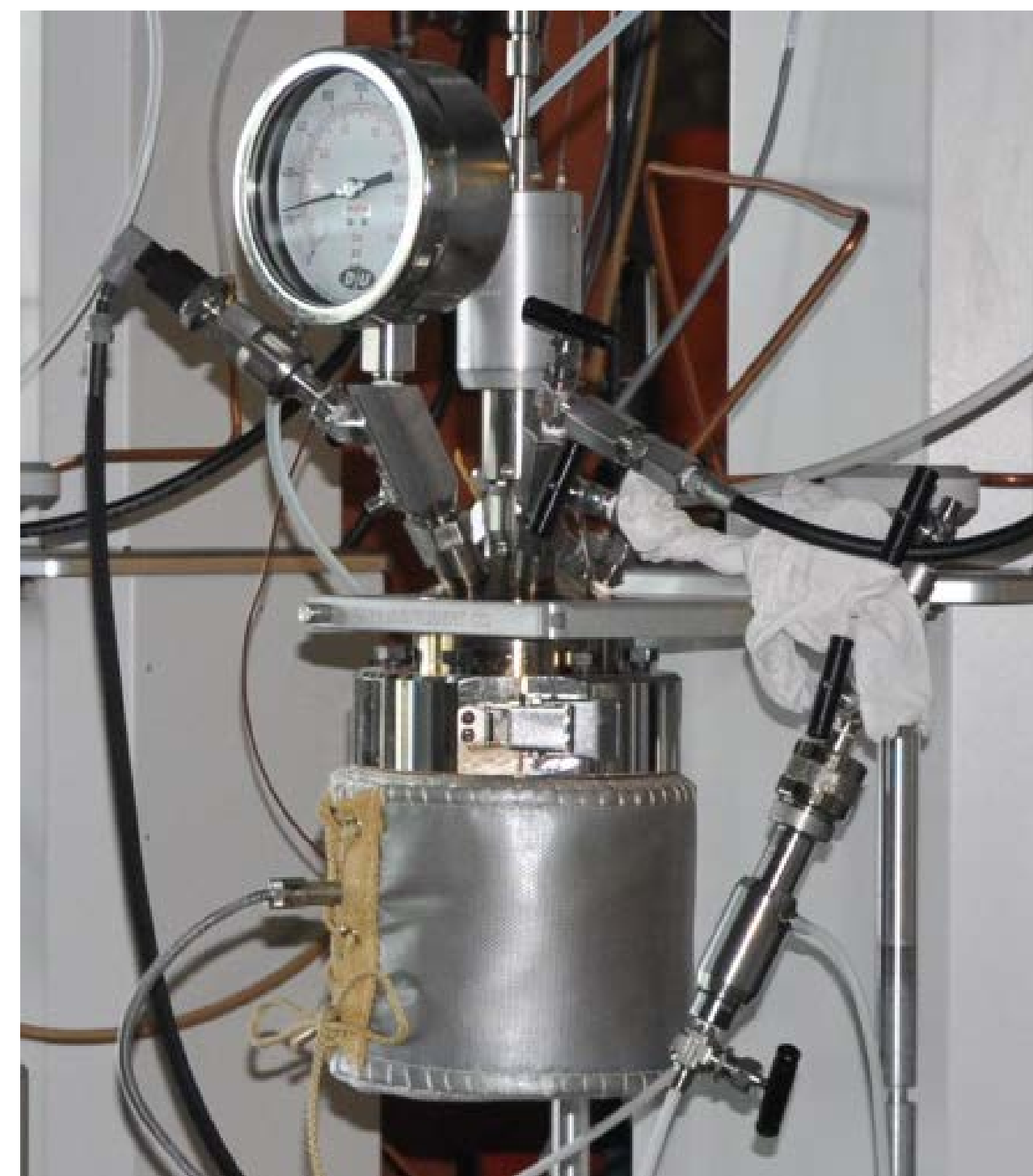
Bench-top, 1-L Parr stirrer reactor set used for Water-rock interaction experiments
