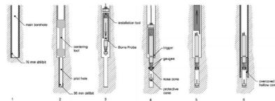
Figure 1: General steps in overcoring illustrated by the Borre probe (from Hakala et al., 2003).
