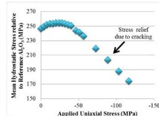
Hydrostatic stress vs applied uniaxial stress for 1st round sample (left) and microstructure of material (left)
