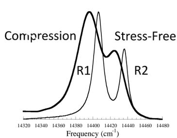
The peak shift gives the mean hydrostatic stress in randomly-oriented alumina.
