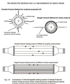
Fig. 1-5 Comparison of interchangeable loading sections of Serata Probe for choice of high accuracy stress measurement by single fracture method or faster property measurement by double fracture method
