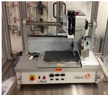
Installed slot-die coater
