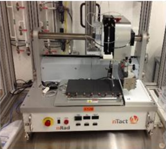
Installed slot-die coater
