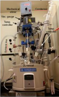
Installed Scale Reactor
