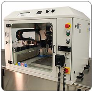
Installed spray coater
