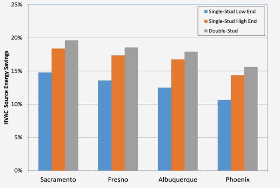
HVAC source energy savings of 11%-18% are projected for 2x6 wall types.
