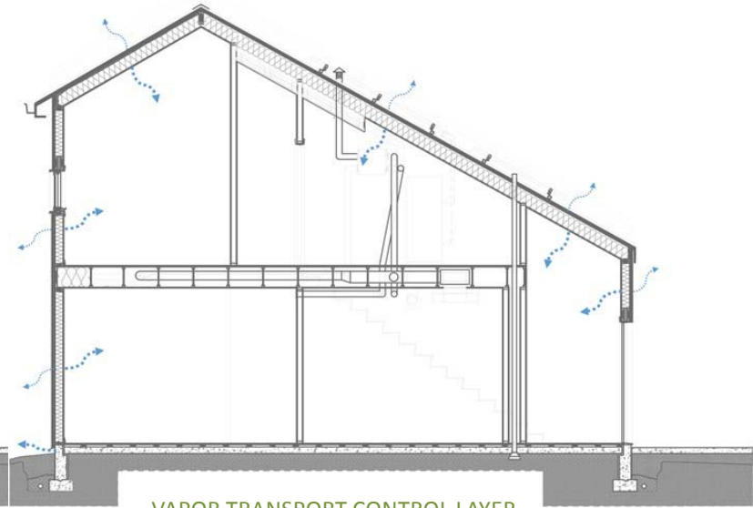
VAPOR TRANSPORT CONTROL LAYER
