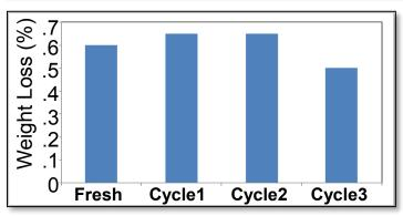
Weight loss of fresh and regenerated catalyst in oxidative furnace shows the efficacy of carbon removal
