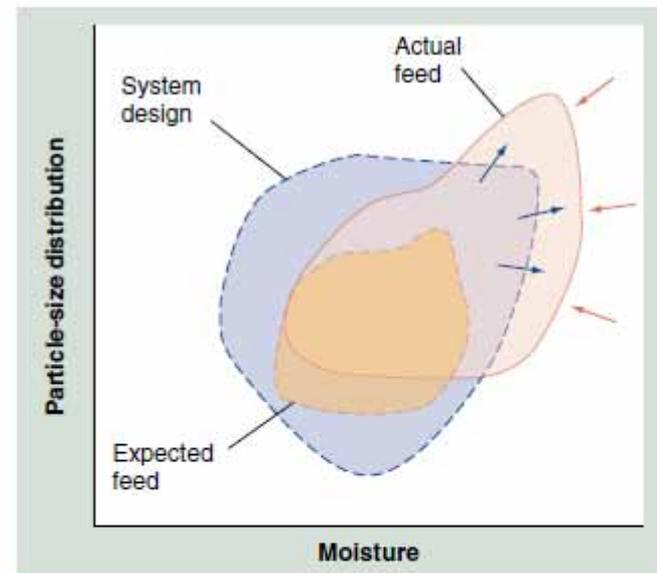
**Figure 5. The combined approach for solving biomass handling and feeding problems through improved system design to expand equipment performance and improved preprocessing operations that constrain feedstock properties to conform to specifications.**
