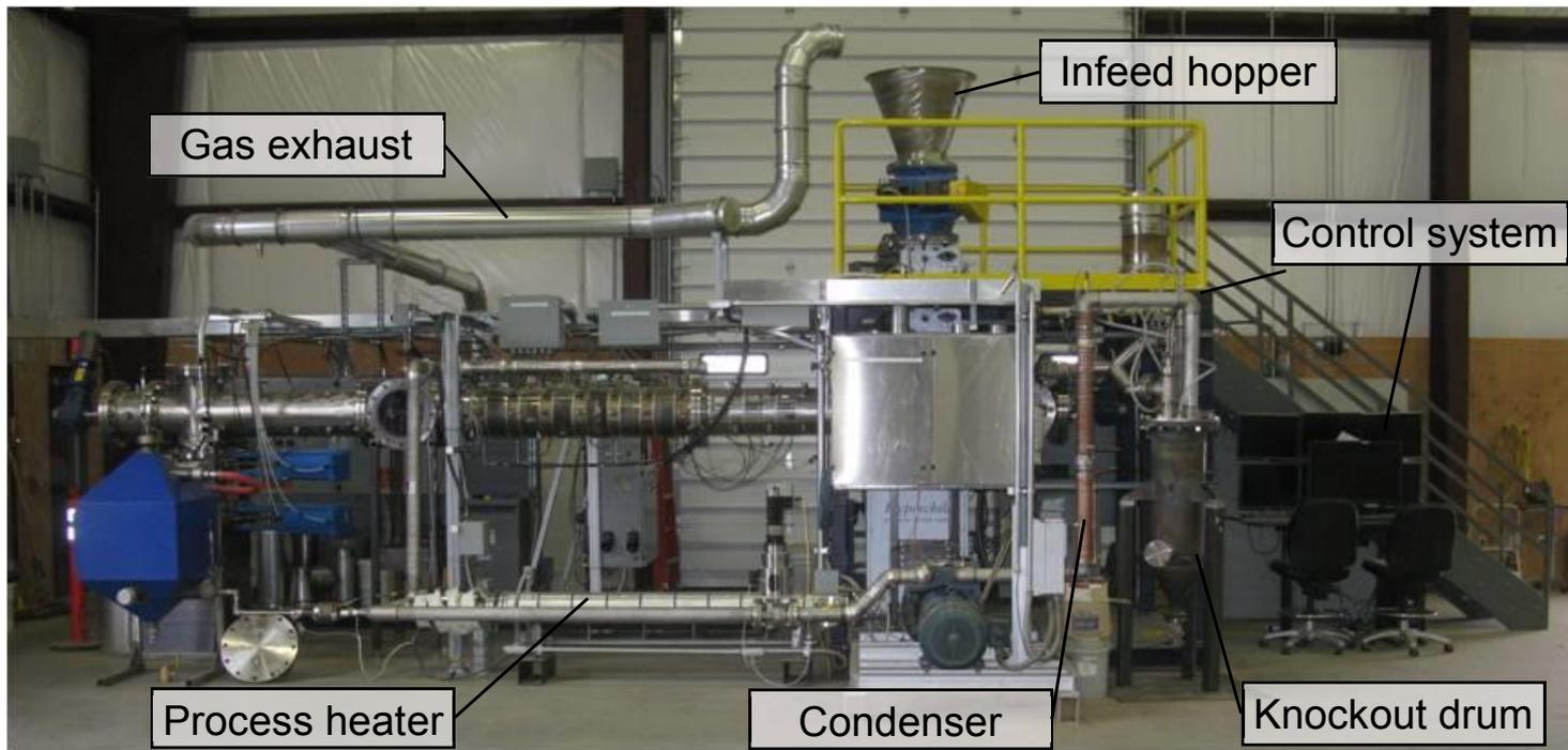
**Continuous feed thermal treatment system at INL (20 kg/hr)**
