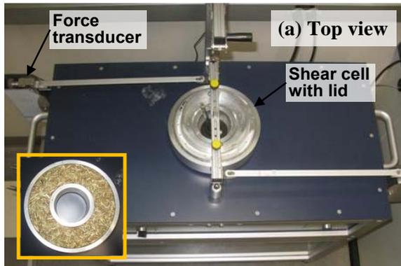
Schulze ring shear tester. Inset: filled cell.
