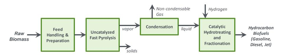
Biomass is rapidly heated in a fluidized bed reactor to yield vapors, which are condensed into a liquid bio-oil. This bio-oil is subsequently hydroprocessed to produce hydrocarbon biofuel blendstocks.
