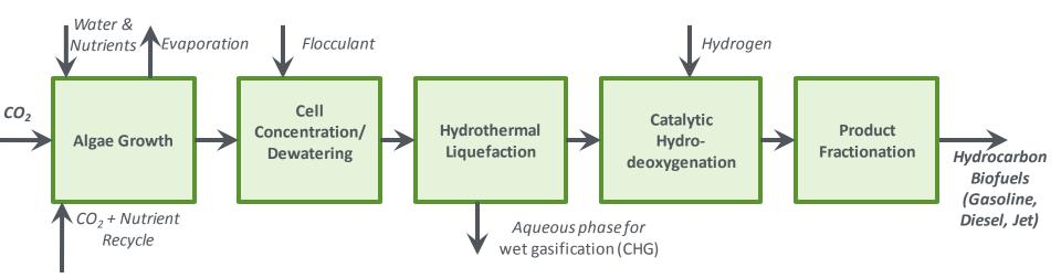
Whole algae cells are treated with heat and pressure to create bio-oil that can be hydrotreated and converted to advanced hydrocarbon fuels.
