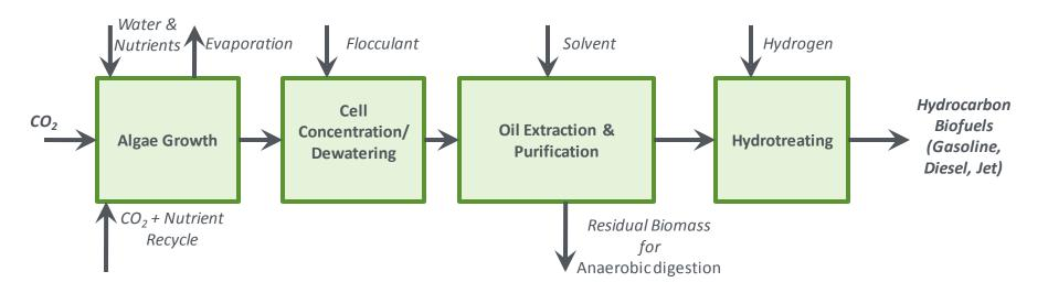
Lipids are extracted from wet algal biomass via high-pressure homogenization and a hexane solvent; the algal oil can then be hydrotreated to produce advanced hydrocarbon fuels.
