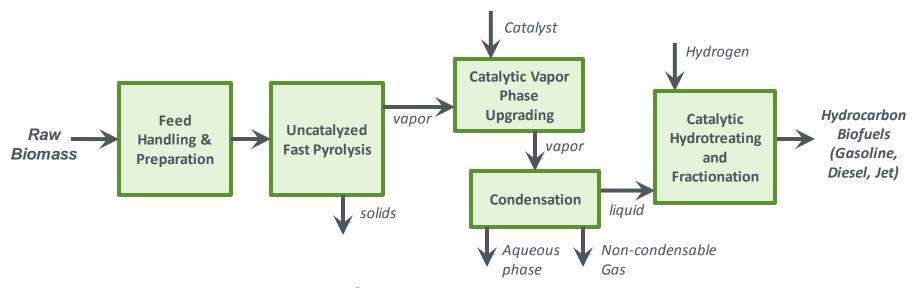
Biomass is rapidly heated in a fluidized bed reactor containing a catalyst to yield vapors, which are catalytically modified and condensed into a partially stabilized and deoxygenated liquid bio-oil. This stable bio-oil is subsequently upgraded to produce hydrocarbon biofuel blendstocks.
