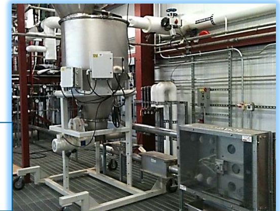
Wet feed hopper and drag tube conveyor
