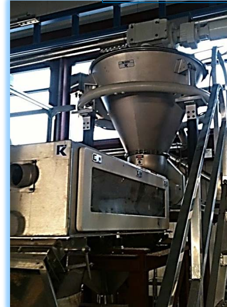
Integrated feed hopper and weigh belt
