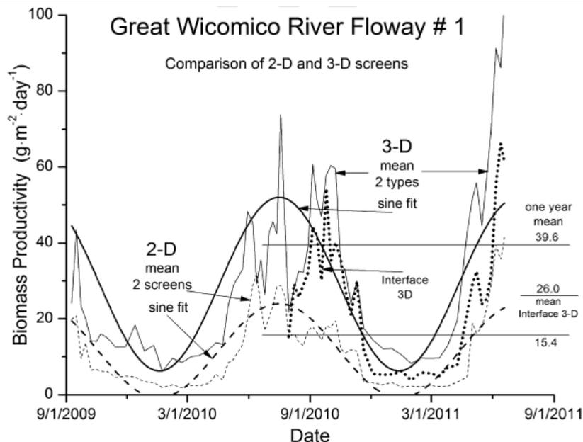
Biomass productivity on Floway #1, comparing 2-D (dashed lines), 3-D (solid lines) and Interface (bold dotted line) growth substrate (screens). The smooth curves are sine functions fit to the two data sets. Note the one-year mean production marked for different screen types (Adey, et al. J. Phycol. 49, 489–501, 2013).
