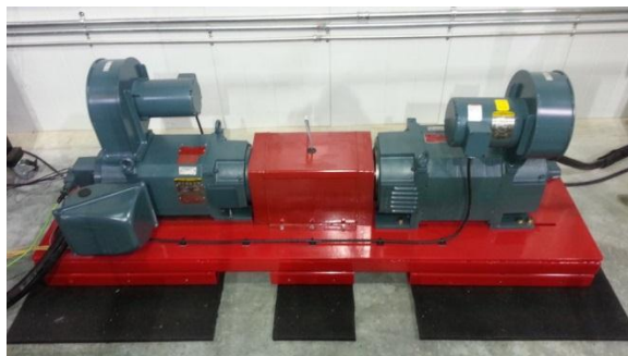
Figure 3-125: The motors, sensors, and dynamometer frame.
