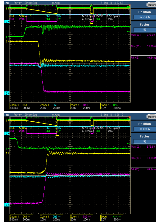
Figure 3-112: HT-3201 turn-on (top) and turn-off (bottom) switching waveforms. (Bus voltage = 600 V, (Inverted) Current = 400 A).
