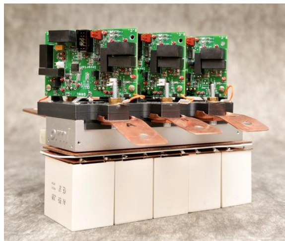
Figure 1-5: 10 kW SiC inverter prototype.
