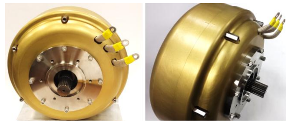
Figure 4-25: Proof-of-principle prototype assembly of novel synchronous reluctance motor.
