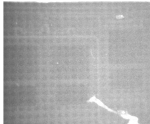
Figure 3-104: "River Void" in Substrate to Manifold Joint.
