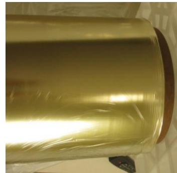
Figure 3-91: Image of a PEI film roll with wrinkles and crease.
