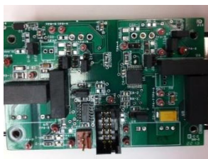
Figure 3-29: Gate driver board for a single-phase power module.
