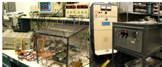
Figure 3-60: Test setup for the 6.6 kW SiC-based isolation charger converter.
