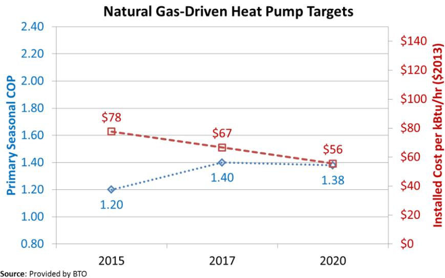
**Figure 1-9: Cost and efficiency targets for natural gas -driven heat pumps**
