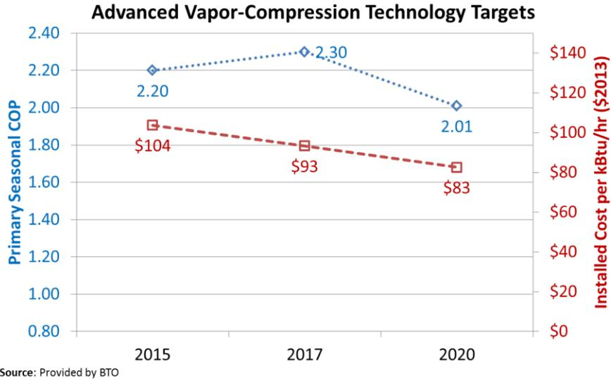
**Figure 1-7: Cost and efficiency targets for advanced vapor-compression technologies**
