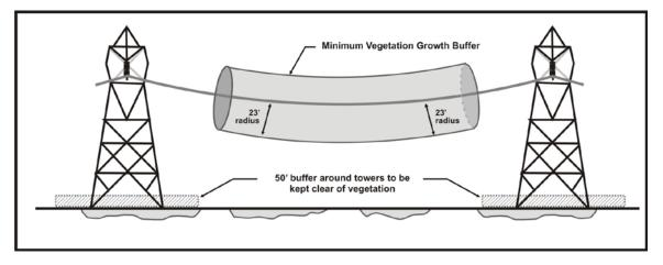
Figure 2-3. Buffered Vegetation Management Approach for 230-kV Line
