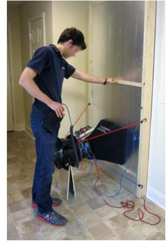
Concept for testing airflow through a door frame (left) and actual test in progress (right).
