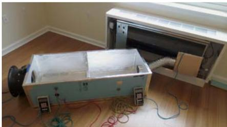
To test the airflow through the PTAC fresh air kit, the team used a custom device that combines a powered capture hood and an orifice plate. The pressure on the PTAC fresh air fan is affected by the conditions in the apartment—exhaust fans, PTAC fresh air fan, and blower fan. As the pressure changes, so does the flow the fresh air fan delivers.
