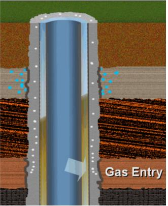
Develop laboratory and modeling techniques to evaluate shallow gas effects on well cement hydration
