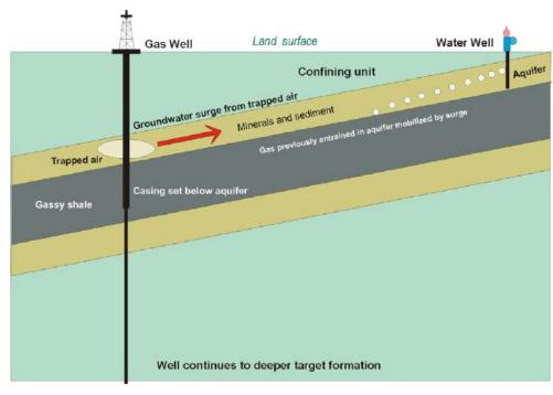
Schematic hypothesis of how shallow gas may migrate during drilling Potential for natural processes to mitigate groundwater issues (*natural attenuation – new*)
