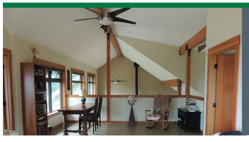
Large south-facing windows allow any available sunlight to warm up the concrete flooring on the first and second floors. These thermal mass floors absorb solar energy during the day and radiate the heat into the space throughout the night. Deep overhangs block out high summer sun and an innovative ventilation system that uses multiple timered exhaust fans to pull air into and out of the house can remove unwanted heat during the early morning hours in the summer.
