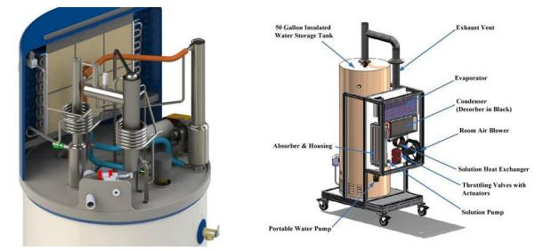
Figure 4-3: Absorption HPWH Architectures (left: NH<sub>3</sub>-H<sub>2</sub>O cycle, right: H<sub>2</sub>O-LiBr cycle)<sup>21</sup>
