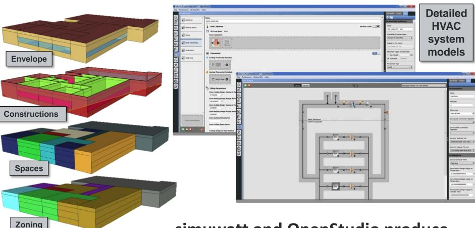
simuwatt and OpenStudio produce the complete model needed for rigorous energy analysis
