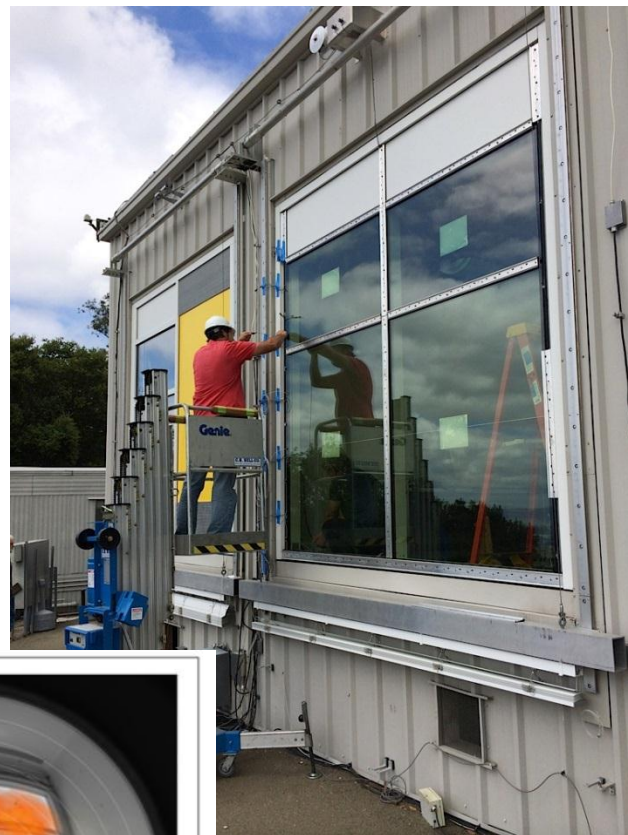
Testbed exterior with EC windows (above) Time-lapsed field measurements of glare in LBNL windows testbed (left)
