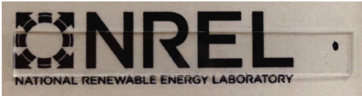
Image of Vacuum Capsules Deposited using Dip Coating, demonstrating virtually no visual degradation.
