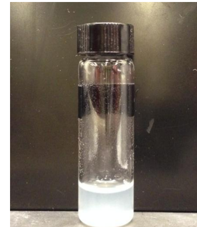
Image of vacuum capsules in water (4 mg/ml) used for dip coating
