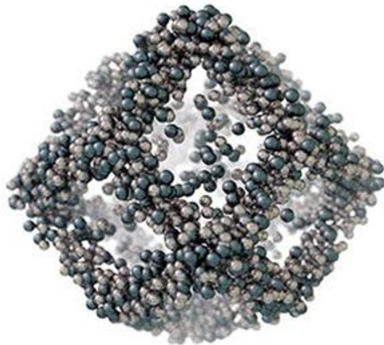
*New nanoframe catalysts developed with mass activity >30X higher than Pt/C catalysts in RDE testing (BES-EERE collaboration)*
