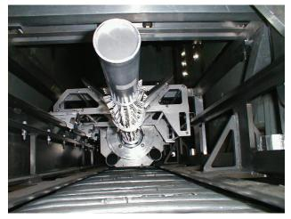
Exhibit 4-5: NuMI Target Module Being Removed from Chase.
