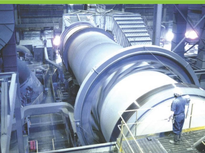
Process lines in the Minntac plant serve kilns that heat a mixture of taconite powder and clay at 2,450°F to create taconite pellets. After installing a high-efficiency burner in one of their process lines, Minntac saved \$760,000 and 95,000 MMBtu in natural gas.
