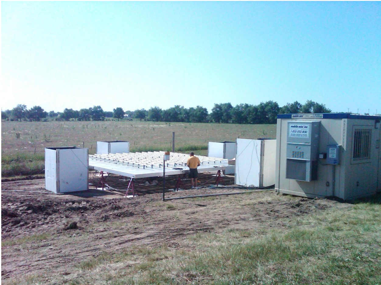
Figure 2.3. The WFIP 449 MHz wind profiling radar located at Buffalo, ND. The four white enclosures house the RASS loudspeakers, and the small portable building contains the computer data acquisition system and communication equipment.
