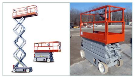
Figure 1-1. Examples of extended and unextended Skyjacks
