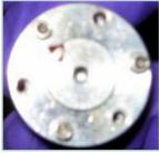
three screws was inconsistent with the safety review expectations and posed an increased risk of the canister seal failing
