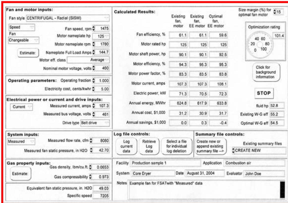
Looking at the printout of the FSAT run with “Measured” data, we see that the system has a very high optimization rating of 101.4 %. This means the fan itself is performing well, and is efficiently producing the flow and pressure measured. This does not mean that the fan is well matched to the process, however.
