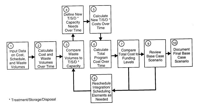
Figure C.5 Steps in Developing Base Case Scenario
