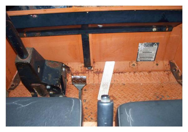
Figure 9: Cart Accelerator Pedal
