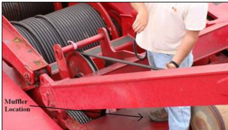
Figure 3-1: Crane Muffler Location
