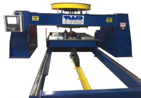
Figure 2. Setup of a high-speed FSW machine at TWB Company LLC in Monroe, Michigan.
