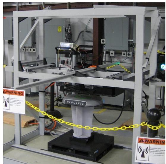
Figure 1. Wireless PEV charger coil positioning measurement setup testing the Evatran PLUGLESS™ wireless charging system at INL. Horizontal alignment occurs through moving the secondary coil mounted in the center of the metal frame relative to the primary coil mounted on the pedestal on the black base. The coil-to-coil gap is the vertical distance between these two parts.
