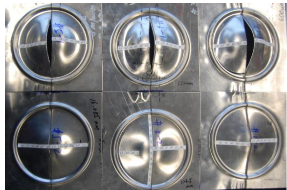
Figure 1. Formability tests on dissimilar thickness welded panels demonstrating weld parameter variation on quality and post-weld formability.
