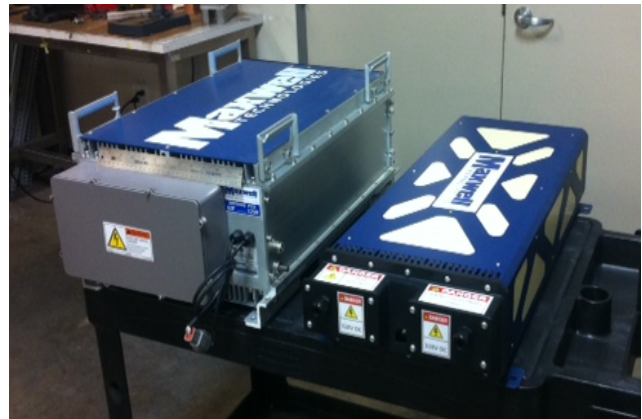
Figure 1. The new asymmetric ultracapacitor pack, on the right, contains almost three times the energy yet it is less than half as large as the current product, shown on the left for comparison.
