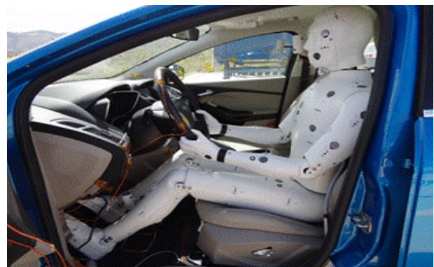
Figure 1. HVAC manikin test in the Ford Focus EV.
