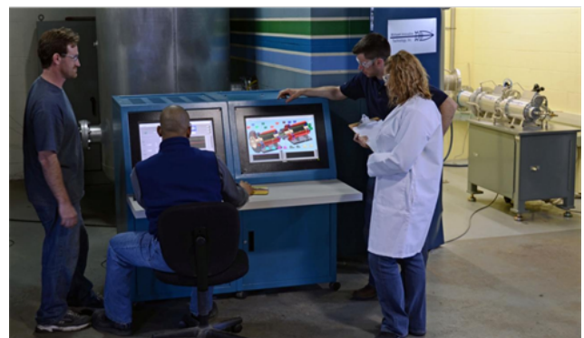
Figure 1. The operation of the single-stage centrifugal compressor in the new test chamber at 60,000 rpm.
