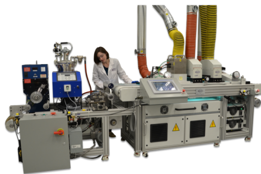
Figure 2. 10" wide slot die press with UV curing shrinks the length of electrode coating operation to 4.2 meters. This eliminates coating ovens and solvent recovery from electrode coating processes.
