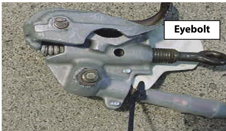
Figure 6: Eyebolt of "cold-end" clamp where victim attached the lanyard snap hook to loosen the ground connection.
