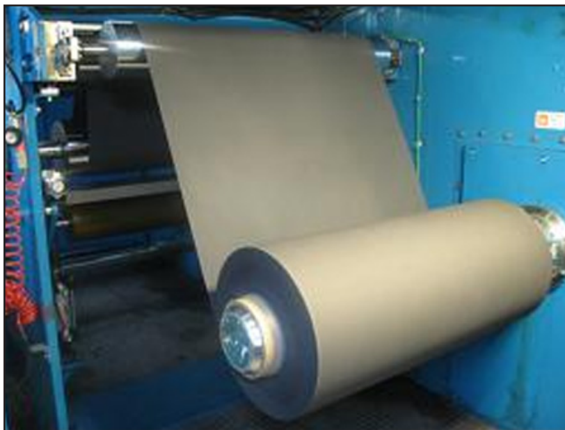
Ballard's Continuous GDL Roll Manufacturing
