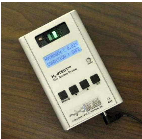
IOS's Prototype H 2 -dTECT Hydrogen Sensor
