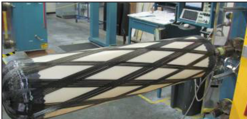
Quantum's Hybrid Manufacturing Technology for Pressure Vessels
