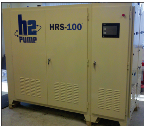
H2Pump's 100 kg/day Hydrogen Recycling System
