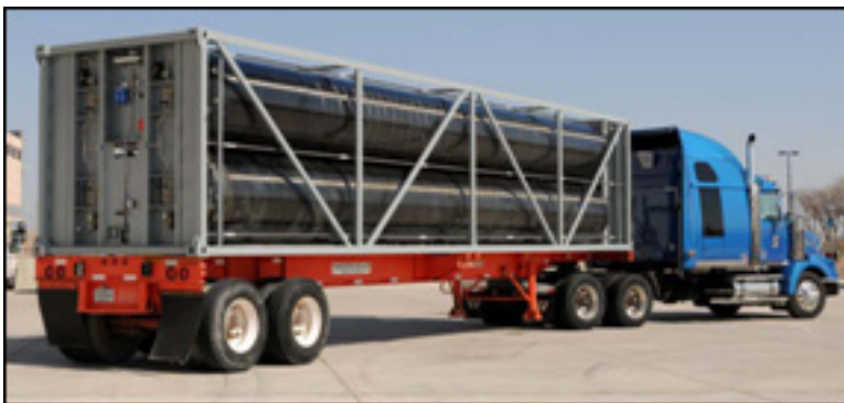
Lincoln Composites' 3,600 psi TITAN™ Tank and Frame System
