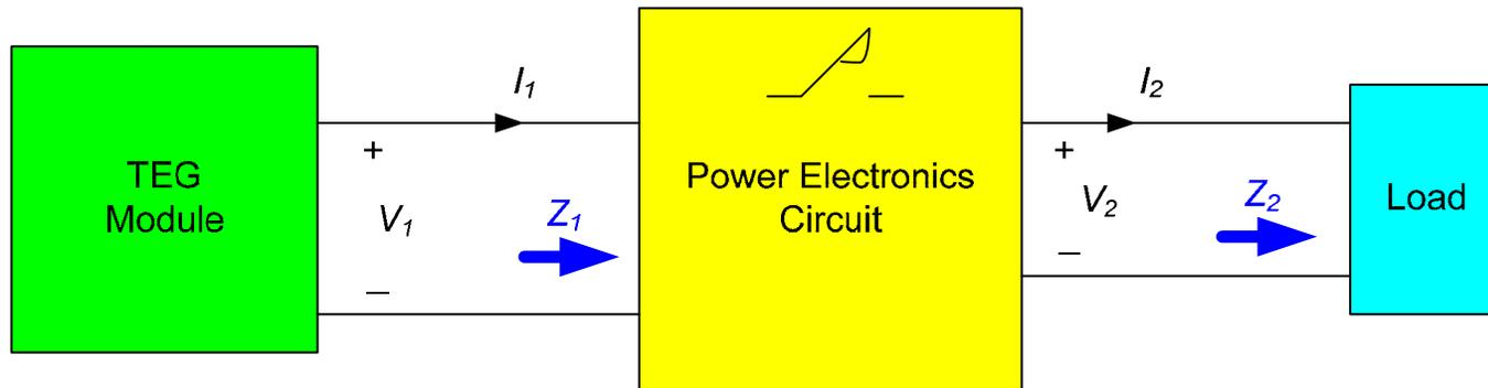
**Developing power electronic circuit as an interface between TEG module and load with the features of:**
