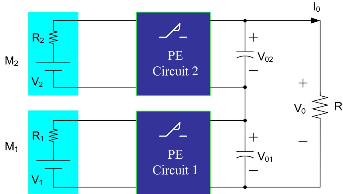
**A power electronic circuit is designed for each TEG module and features functions of:**
