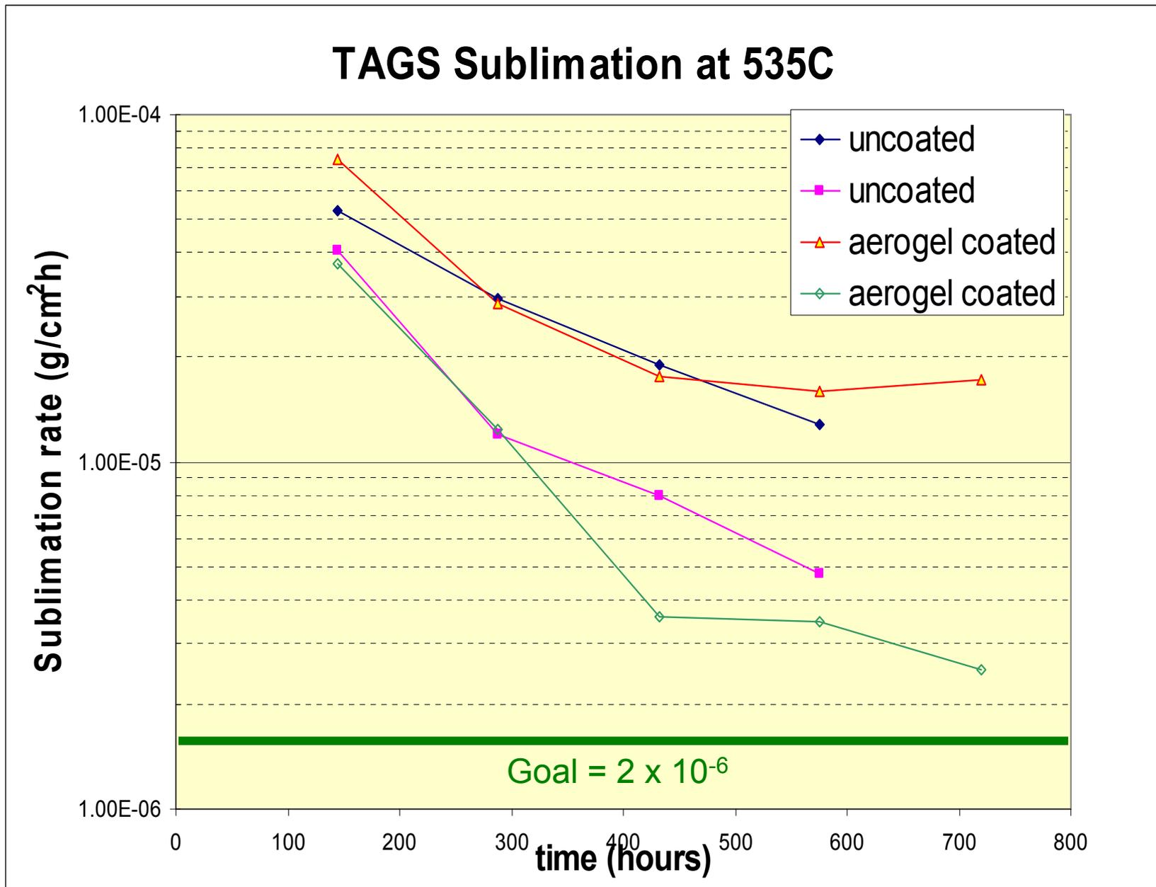
❖ Aerogel suppressed sublimation by a factor of 10 and is approaching the 10 years of operation goal at 535C
