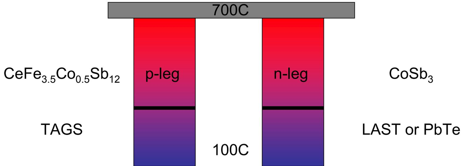
**Option 1:** LAST for cold stage of n-leg (525C interface) = 14.80% efficiency
