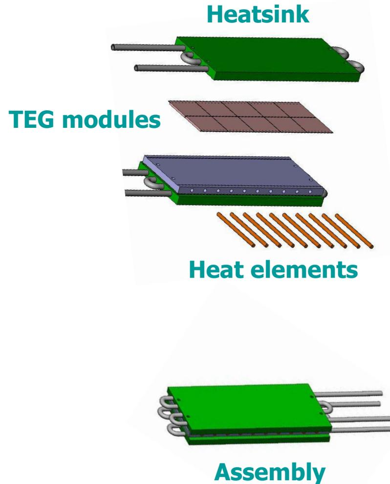
➤ A heat exchanger capable of 100 W electrical power output has been fabricated and Tested.
