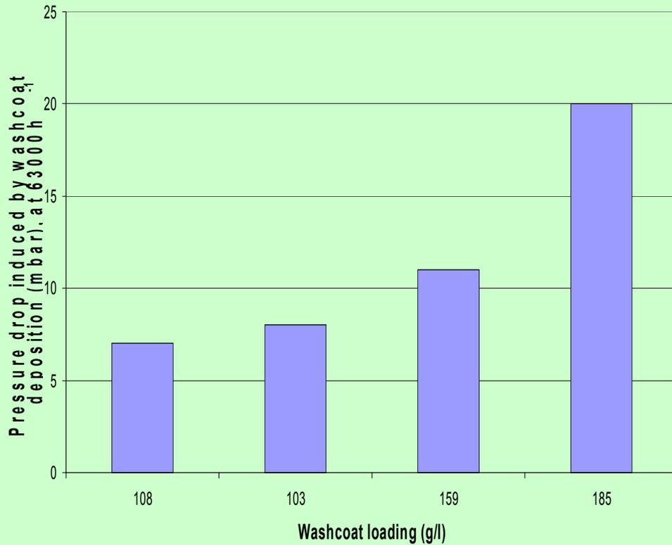
Pressure drop as a function of washcoat loading
