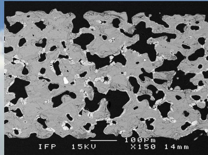
SEM pictures of a core loaded with 159 g/l catalyst
