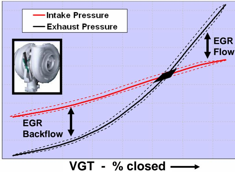
Actuator Internal Position Feedback & Trim Significantly Reduce Emissions Variability
