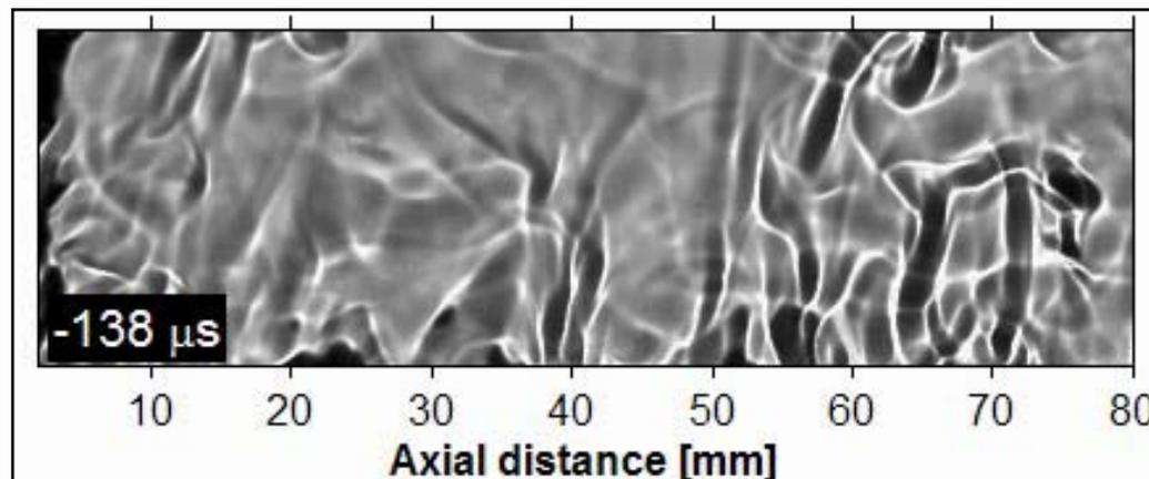
High-speed shadowgraph, showing stagnant, low-velocity gases near injector after the end of injection, while downstream gases have higher velocities.
