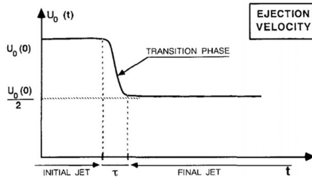
Figure 1. Typical temporal evolution of the ejection velocity.
