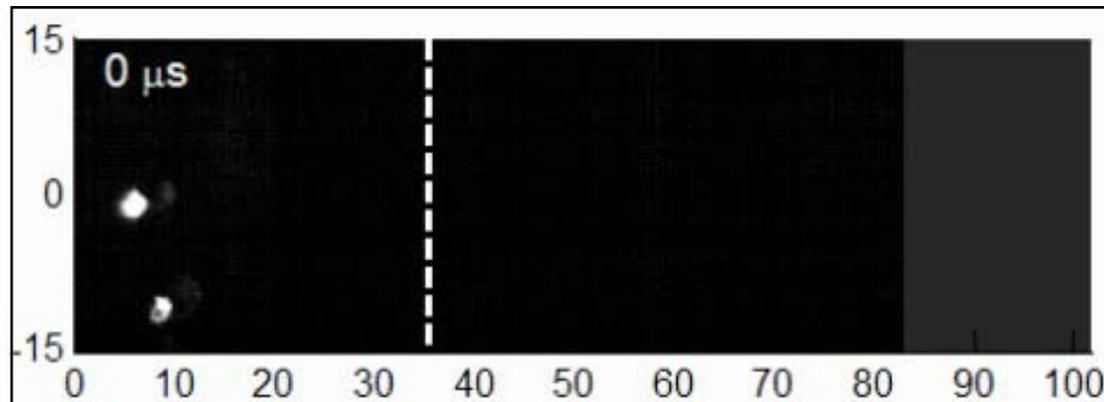
High-speed movie of combustion chemiluminescence, showing that combustion does not propagate upstream after end of injection
