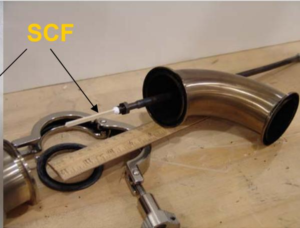
SCF assemble inserted in S.S exhaust elbow
