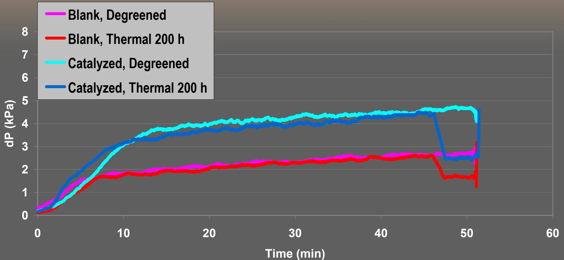
➤ Thermal aging of 200 hours has only a minor impact on pressure drop
