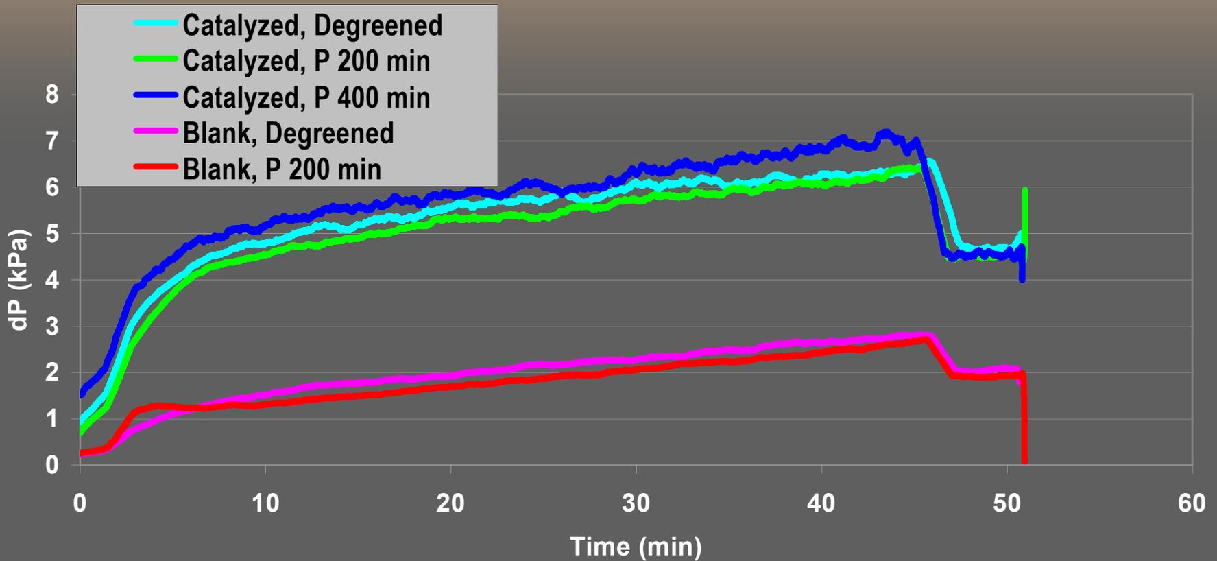
➤ Chemical aging by phosphorus has only a minor impact on pressure drop
