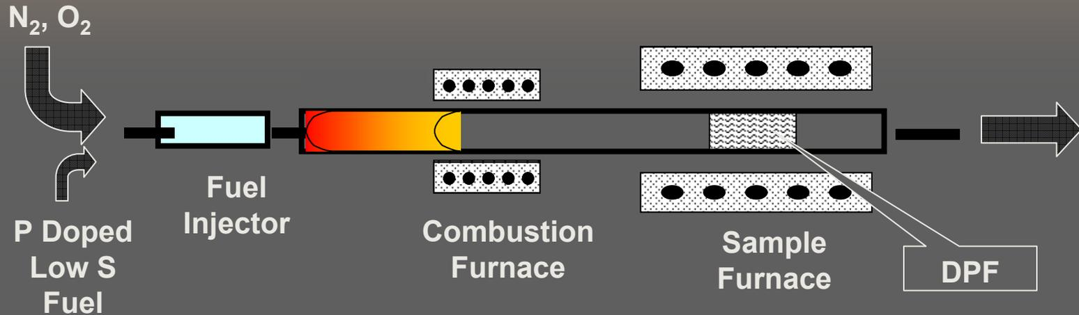
**Phosphorus (P) source:** 1% (TCP) Tri-Cresyl Phosphate  $[(4\text{-CH}_3\text{C}_6\text{H}_4\text{O})_3\text{PO}]$
