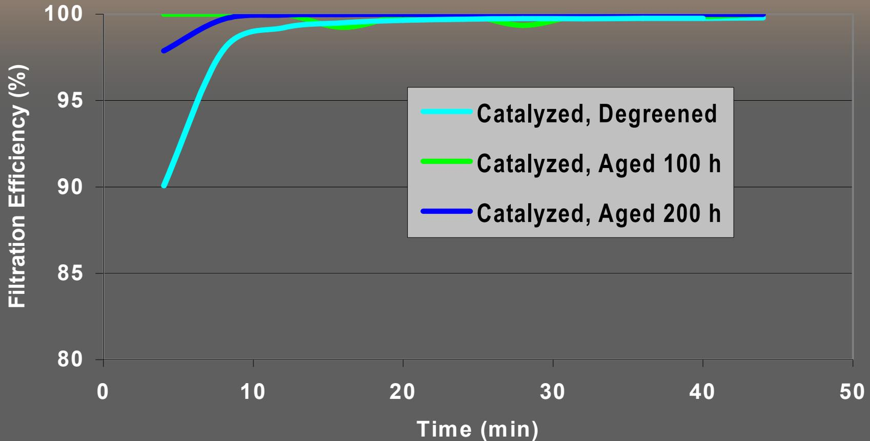
➤ Thermal aging of 200 hours has a minor impact on filtration efficiency
