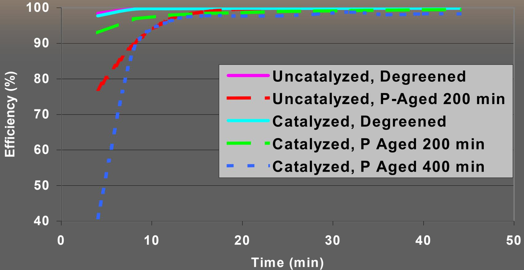
➤ Phosphorus aging decreases the filtration efficiency of diesel particulate filters
