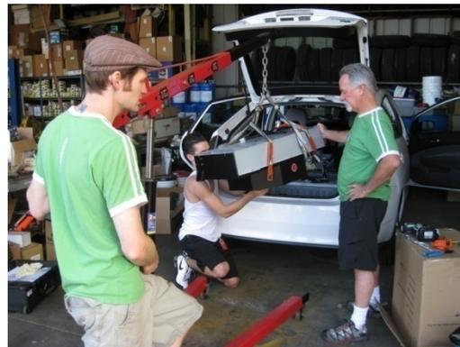
**Figure 2. Green Gears PHEV conversion shop converting a Hymotion Prius at the Maui Electric Company fleet shop.**
