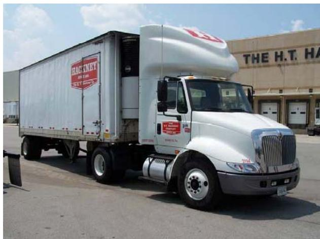
**Figure 1. Typical Class-7 H.T. Hackney Delivery Truck with Non-Refrigerated, Refrigerated, and Frozen Compartments**
