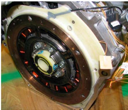
Figure 4. Mounted ICE-IMA Torque Sensor
