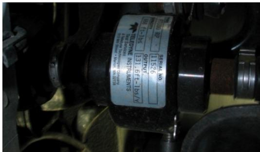
Figure 5. Image of Half Shaft Torque Sensor Mounted on Axle
