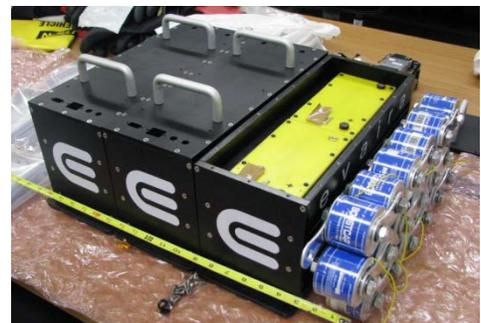
**Figure 3. Three 45-V/30-Ah Sub-System Gold Peak Modules (72 cells each — 12S/6P each)
