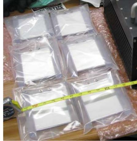
**Figure 4. Gold Peak 5Ah/3.8v Single-Cell Test Articles in Lexan Frame with Robust Terminals for Test Fixture**
