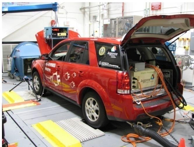
Figure 7. TTR PHEV On Test at the 4WD Dynamometer
