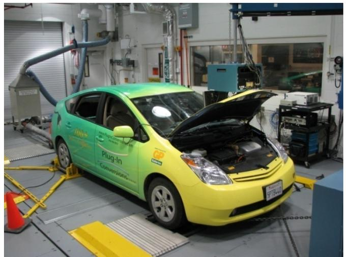
**Figure 9. TTR PHEV On Test the 4WD Dynamometer**
