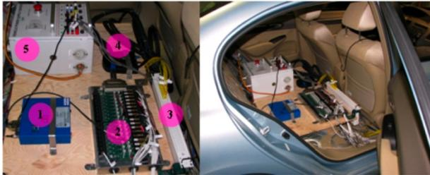
**Figure 1. Vehicle Data Acquisition (DAQ) Layout: 1 Teledyne Engine Torque Sensor, 2 signal conditioning board, 3 NI Thermocouple PXI, 4, Teradyne OBDII interface, 5 power supply**
