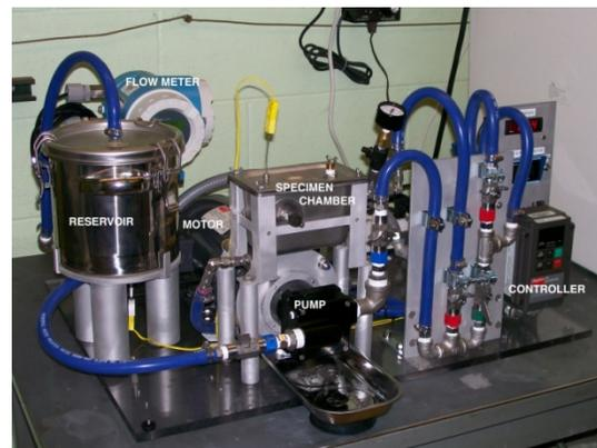
**Figure 1. Photograph of the liquid erosion apparatus**
