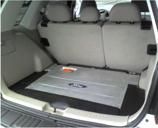
Figure 4. PHEV Battery Pack
