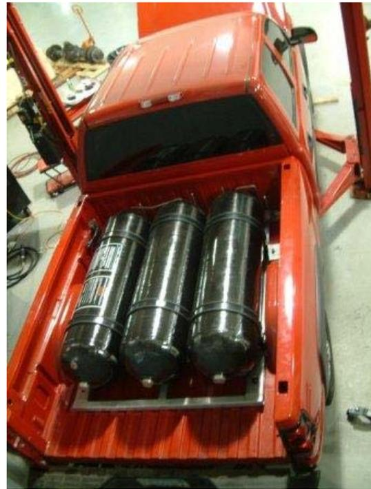
**Figure 1. Dynetek hydrogen fuel tanks in the bed of the pickup.**
