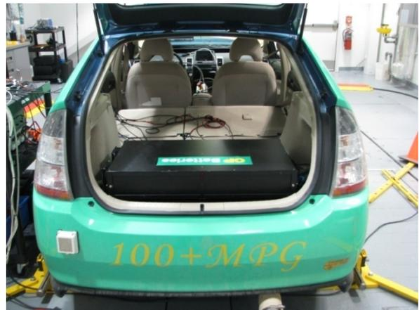
**Figure 8. TTR PHEV On Test the 4WD Dynamometer**
