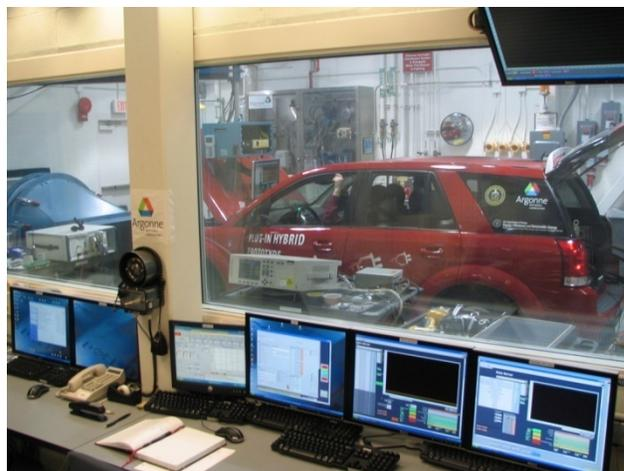
Figure 6. TTR PHEV Testing in the 4WD Dynamometer Cell in Argonne’s APRF
