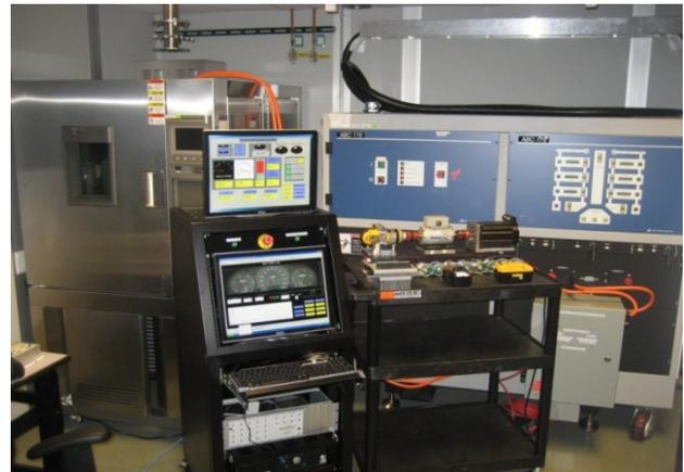
Figure 2. Argonne Battery Systems HIL Test Stand
