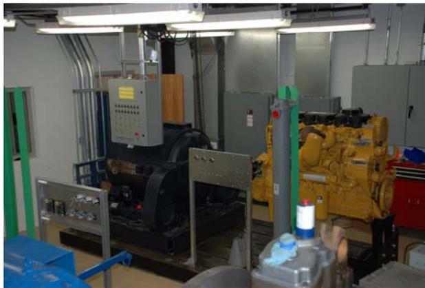
Figure 7. *Photograph showing mounted Caterpillar engine and dynamometer in ORNL engine test cell. The engine will be used for testing advanced component designs and materials.*
