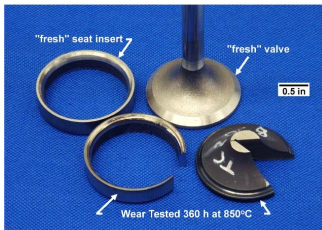
**Figure 2.** Valve and seat components, fresh and Buettner-Rig tested, received by ORNL from Caterpillar for detailed microcharacterization and analysis.
