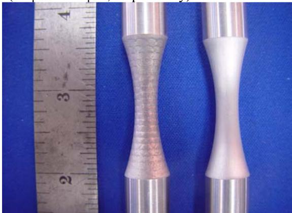
**Figure 1.** Representative image comparing the surface finish of an A354 cast Al laser peened specimen (left) versus a control specimen.
