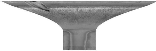
**Figure 8.** Corrected laser-scatter scan image of intake valve I#12 at end of engine test.
