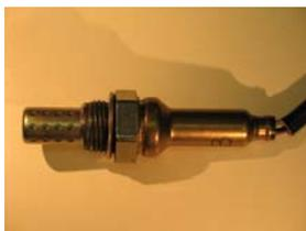
**Figure 9.** Photograph of Pt/YSZ/Au prototype built on a heated substrate and packaged into an oxygen sensor housing.
