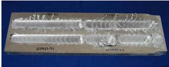
**Figure 9.** Nanotube and Nanofiber FSP trials on 339 plate.
