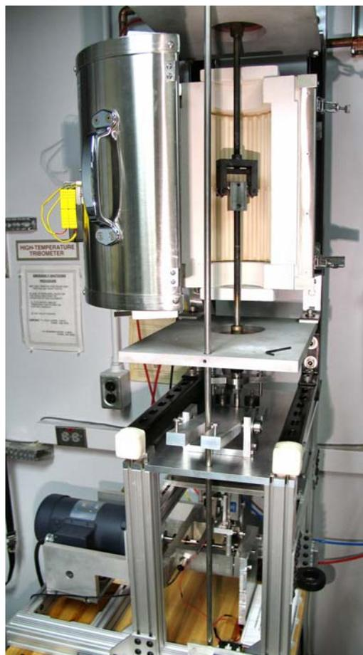
Figure 1. HTRI with the furnace door open to reveal the specimen holders.
