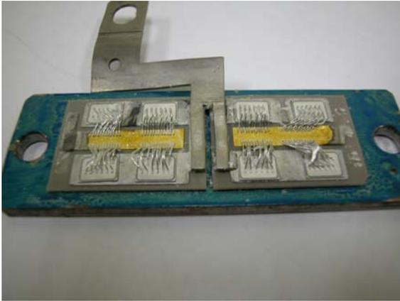
Figure 3. View of the internal construction of the diode module.
