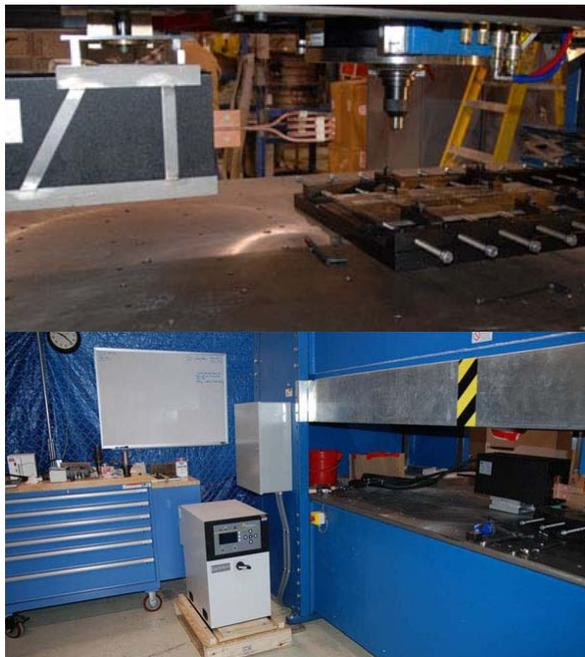
**Figure 10.** 30 Kva induction heating system showing adjustable heat station mounting frame to vary stand off and trailing heat distance (top) and control unit (bottom).
