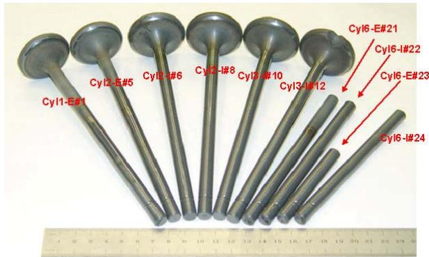
**Figure 1.** Photograph of  $\text{Si}_3\text{N}_4$  engine valves at end of engine duration test.
