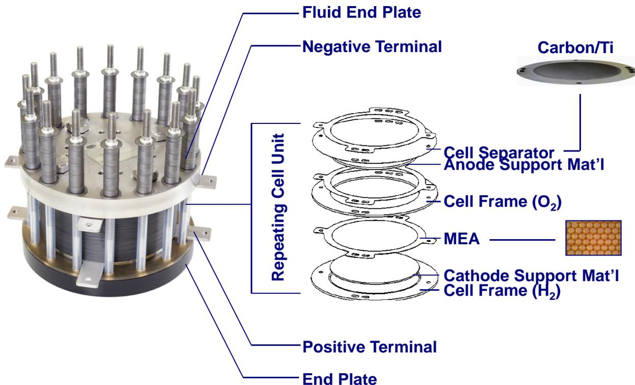
**The repeating cell unit comprises 90% of electrolyzer stack cost**
