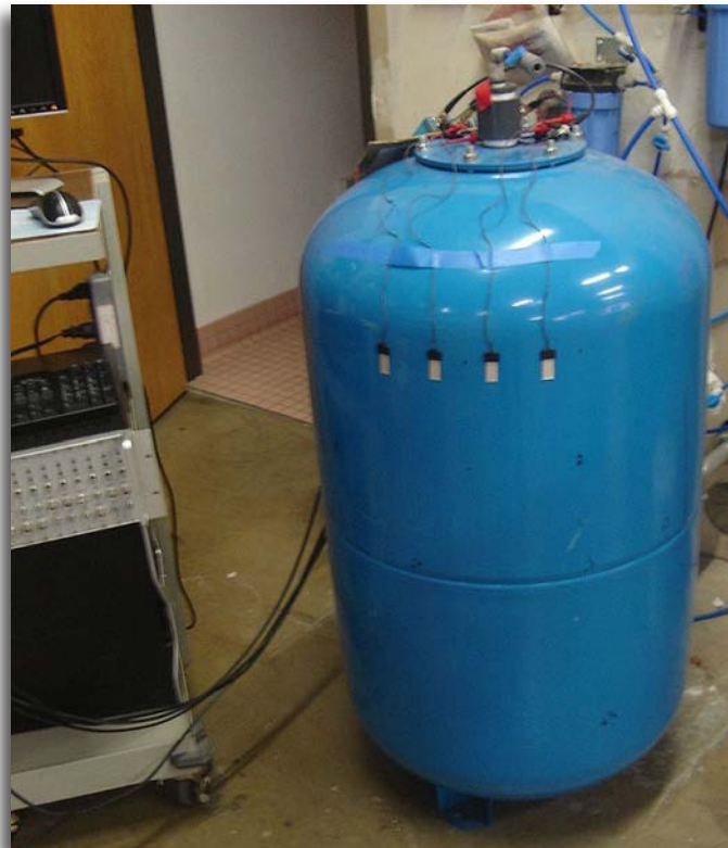
Pressure Tank with Digital Wave's Stress Transducers Attached
