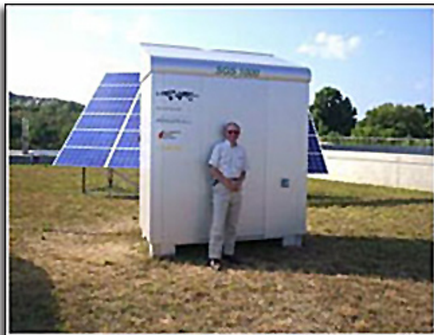
The Avalence Electrolysis Unit with Photovoltaic Array
