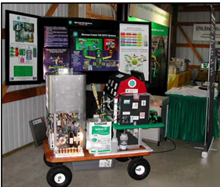
TMI's Multi-Fuel SOFC 1-kW System Operating on Soybean Oil
