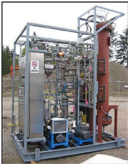
Linde's Prototype Hydrogen Generator Unit
